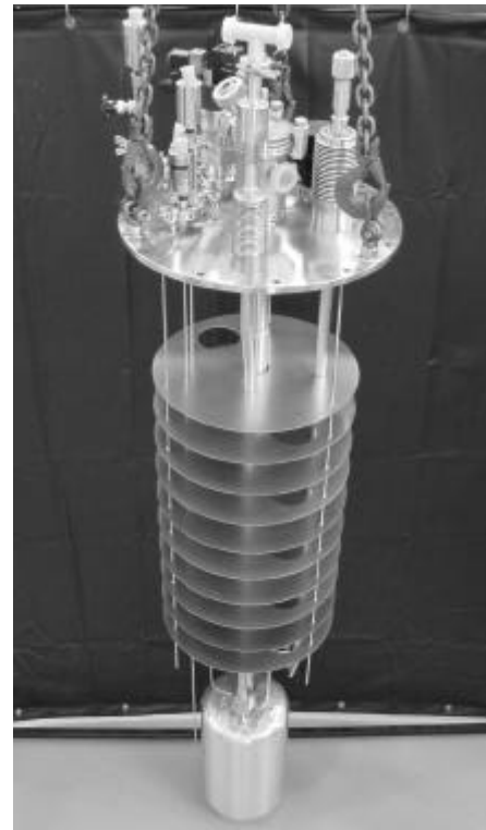
Fig. 2. The test insert ready for assembly into the bucket dewar. The helium vessel at the bottom is approximately 400 mm in length.
