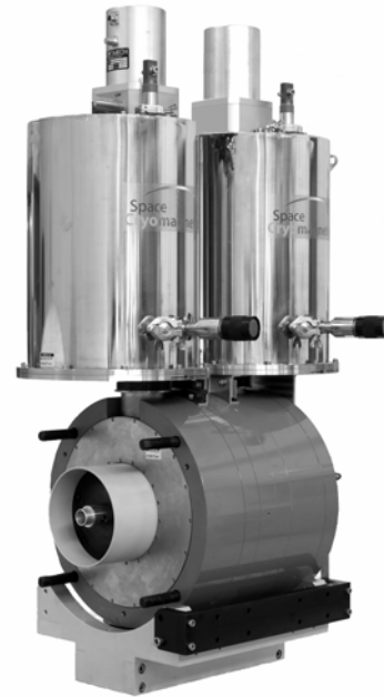
Fig. 5. Two HTS magnets integrated into the iron from the ion source.
