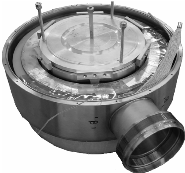
Fig. 4. Assembly of a completed coil into its vacuum vessel.
