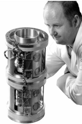
Fig. 6. The completed ADR magnet system, after testing.
