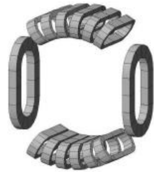
Fig. 1. Arrangement of the AMS magnet coils. The larger coils generate most of the transverse field: the smaller coils constrain the return flux.
